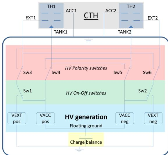
Fig. 1. Simple representation of the PPU architecture
