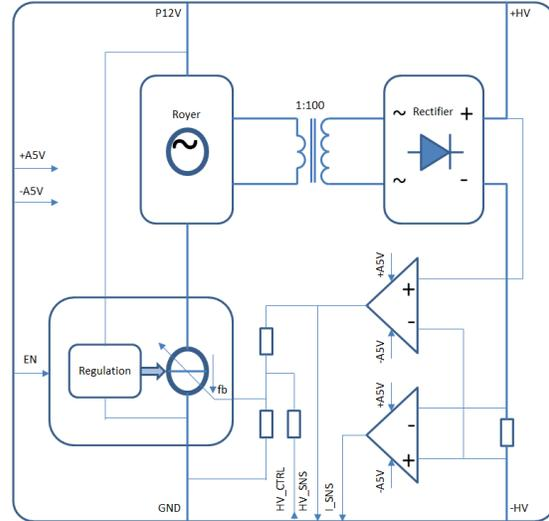
Fig. 2. High voltage generator
