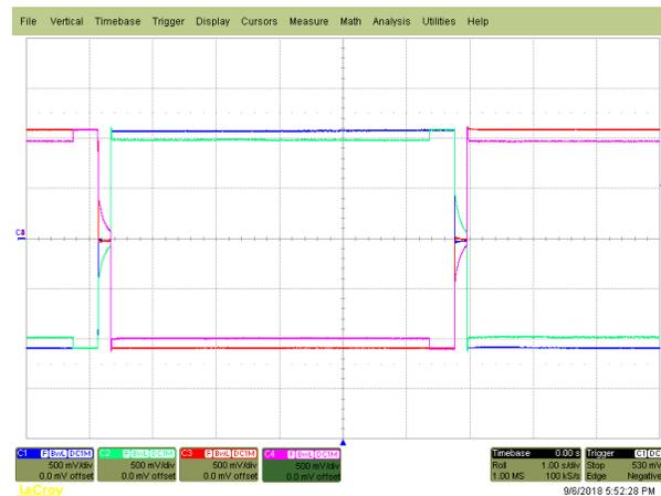
Fig. 5. CTH voltage waveforms in thrust mode
